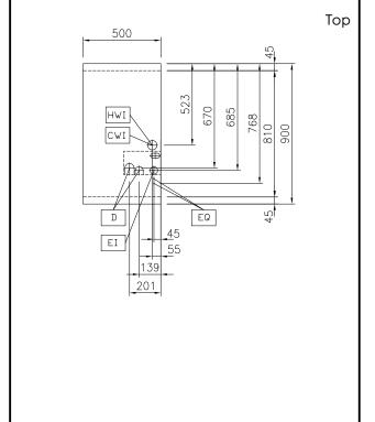
**Electric** Supply voltage: 400 V/3N ph/50/60 Hz Total Watts: 1.5 kW Water: Inlet water line size: 3/4" Incoming Cold/hot Water line 3/4" Drain line size:
